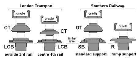
Note the orientation of the bases LOB, LCB and SB with respect to the cradle – the longer dimension of all the bases should align with the timber axis.
